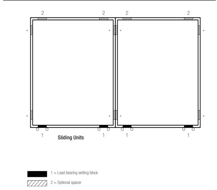
The load bearing setting blocks should be positioned right above the rollers which are positioned at the appropriate distance from the corner.
